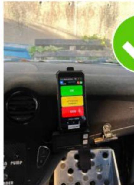
✓ 1/ PLUG the USB cable into the USB port of your car and the USB-C part into the tracker.
